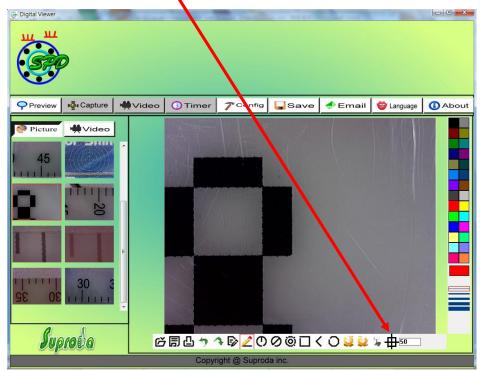
2. Put the Digital Viewer microscope on the Calibration Pattern sheet, you can see the black/white block on the screen.
