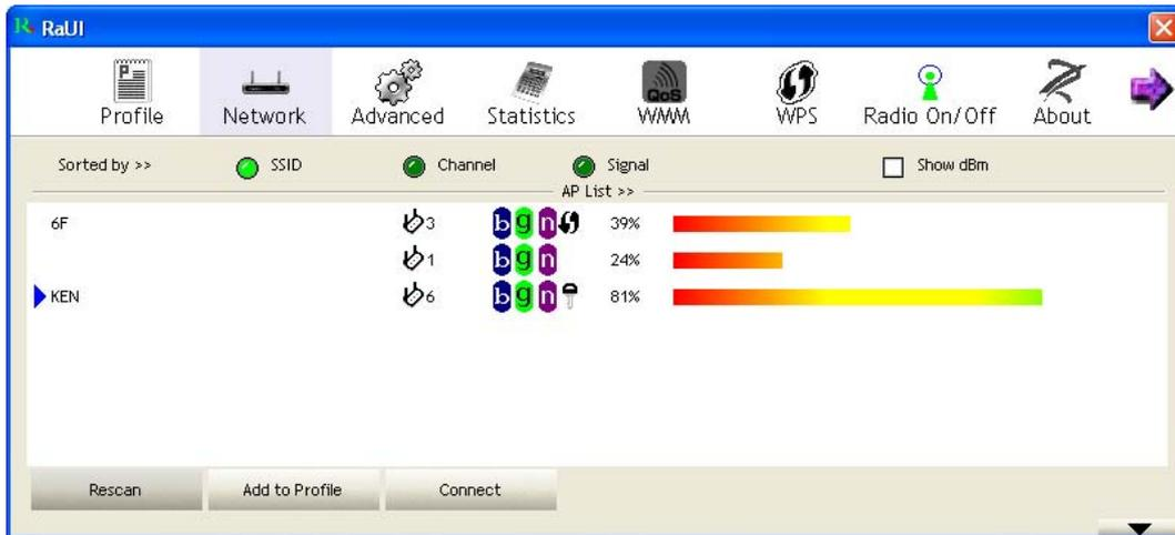
Scan results will be displayed here, please check if the wireless device (access point or another computer) with the SSID you wish to connect is shown here.
