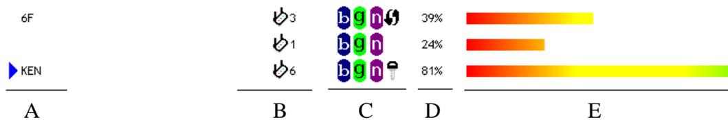
**A** The SSID (Service Set Identifier) of wireless device. If nothing is displayed here, it means the SSID of this wireless device is hidden.
