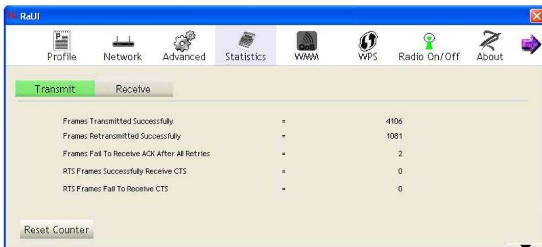
All connection-related statistics is displayed here. You can click 'Transmit' or 'Receive' tab, to view the statistics of transmitted or received packets. You can also click 'Reset Counter' button, to reset the statistics of all items back to 0.
