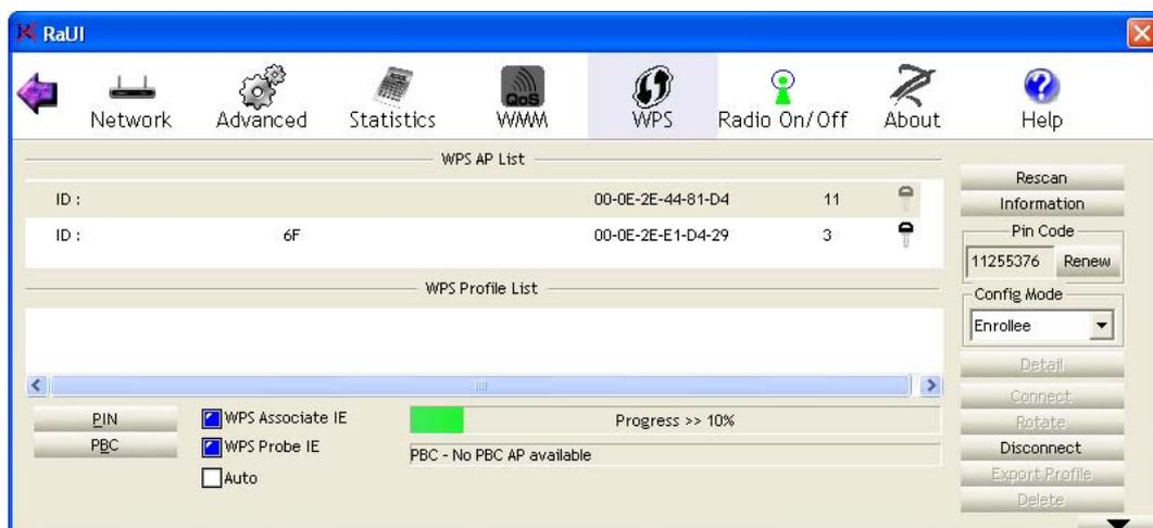
You can click 'PBC' button few more times to try again. When an access point is connected, you can click 'Disconnect' to disconnect your wireless network card from a connected access point, or select another WPS-enabled wireless access point, then click 'Connect' to establish connection to selected access point, if there are more than one WPS-enabled access point found. You can also click 'Rotate' button, and next access point on the list will be selected to establish connection.
