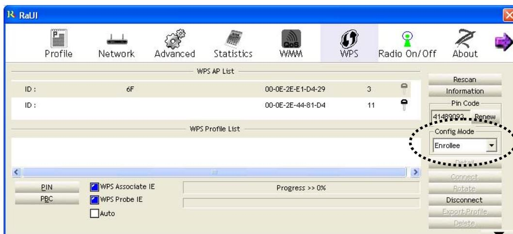
3. Set 'Config Mode' to 'Enrollee', and then push the 'WPS' button on your wireless access point (the button used to activate WPS standby mode may have another name), or use other way to start WPS PBC standby mode as the instruction given by your wireless access point's user manual.
