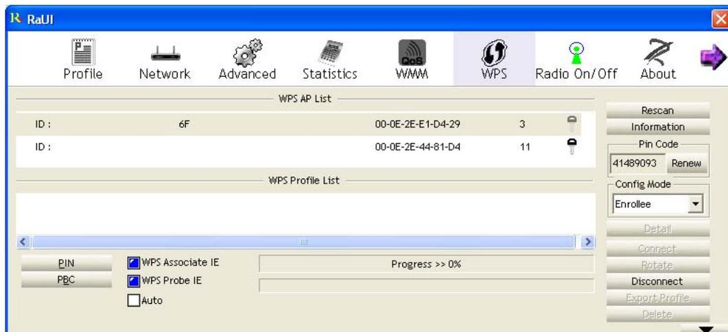
3. The PIN code of your wireless network card is an eight-digit number located at the upper-right position of configuration utility. Remember it, and input the number to your wireless access point as the WPS PIN code (Please refer to the user manual of your wireless access point for instructions about how to do this).
