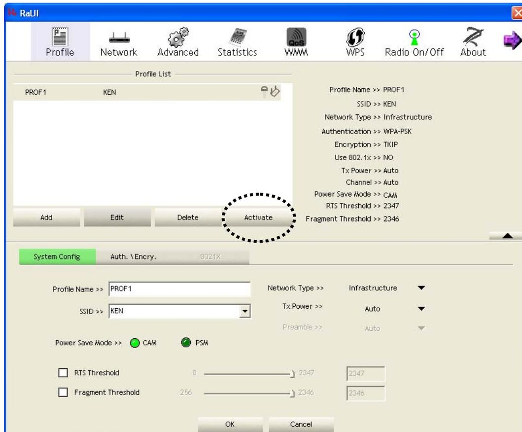
When you selected a profile and click 'Activate' button to activate the profile, a ► icon will be displayed in front of the profile to show that the connection is failed; When the connection is successfully established, a ▶ icon will be displayed.
