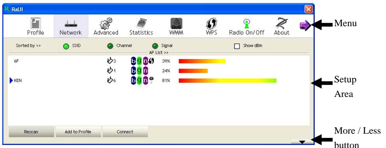
RaUI consists two parts: Menu and setup area. You can select a setup function (Profile, Network, etc.) from menu, and corresponding setup items will be displayed at setup area.
