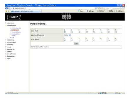
Port Mirroring is used to mirror traffic, RX, TX or TX&RX, from Source port to Destination port for analysis.
