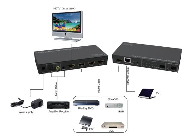
3. Insert the DC side of 5V power supply into the main unit and then connect the AC side of the power supply into the wall outlet.
